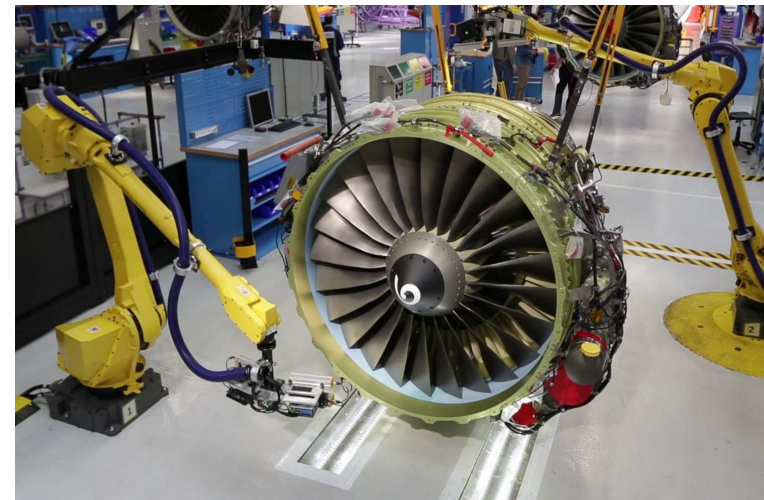
Optically-assisted final inspection
