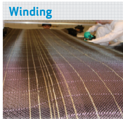
Winded preform on RTM equipment
