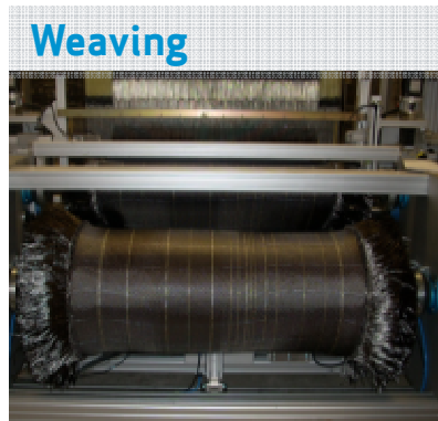
Weaved full scale preform (30 meters length)
