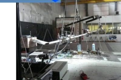
*Wing static bending test in collaboration with ISAE*
